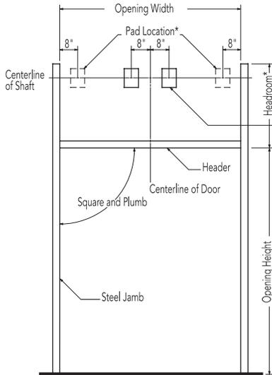
\* Pad Location for additional shaft support brackets for doors over 18'3" wide
