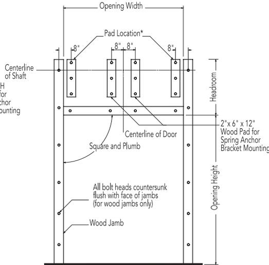
\* Pad Location for additional shaft support brackets for doors over 18'3" wide
